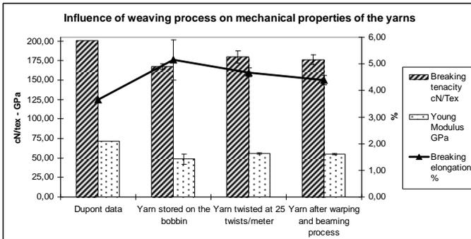
Graph 1: influence of weaving process on mechanical properties of the yarns
