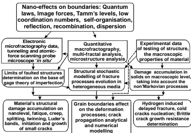
Fig.1 Concept scheme of multiscale modeling
