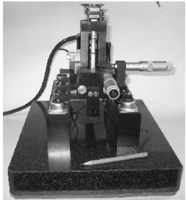
Fig.2 View of the AFM with loading device
