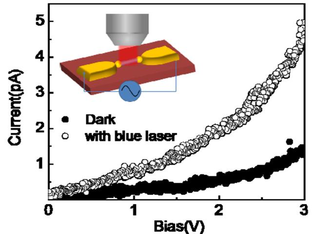
Fig. 2 Room temperature I-V curves with (open circles) and without (filled circles) blue laser irradiation. Inset: schematic drawing of the optoelectrical transport properties measurement setup.
