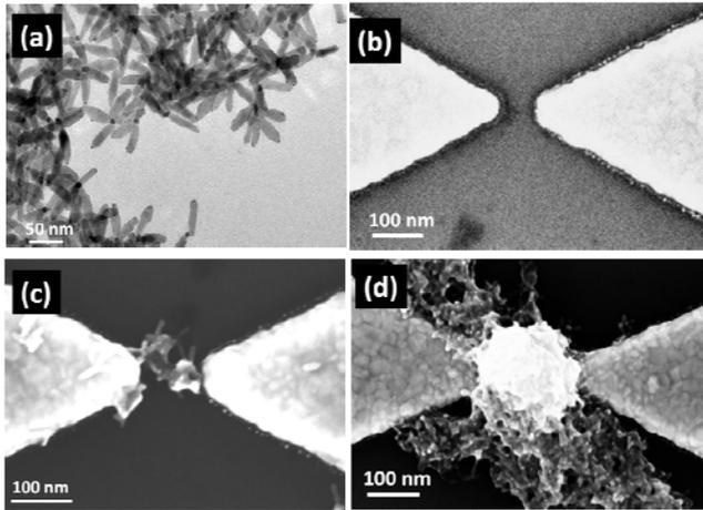
Fig. 1 (a) TEM image of as-synthesized CdSe-Au nanorod networks, (b) SEM image of tip-to-tip electrodes with gap-size about 100 nm, (c) SEM image of a few trapped networks and (d) SEM image of a large quantity of trapped networks in-between planar electrodes.
