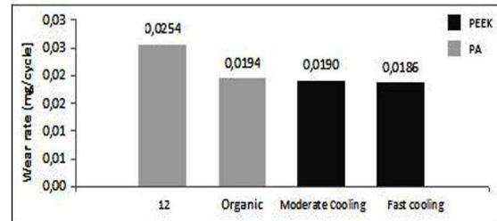
Fig. 4. Wear test results- CETR tribometer
