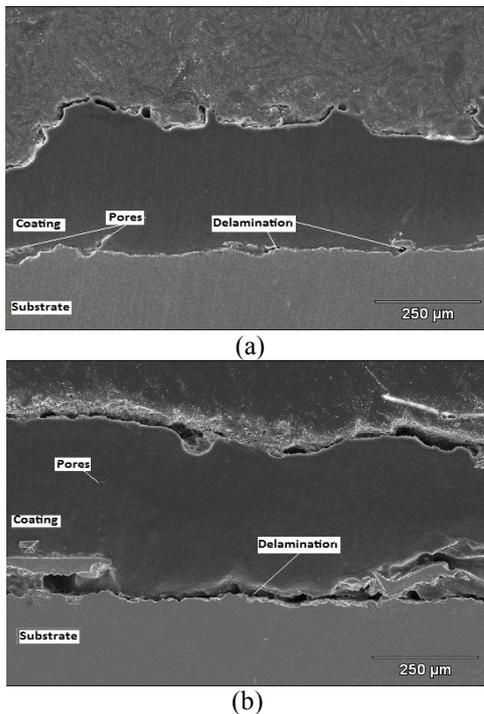
Fig. 2. Cross sectional SEM micrographs of a) PEEK and b) Polyamide coatings
