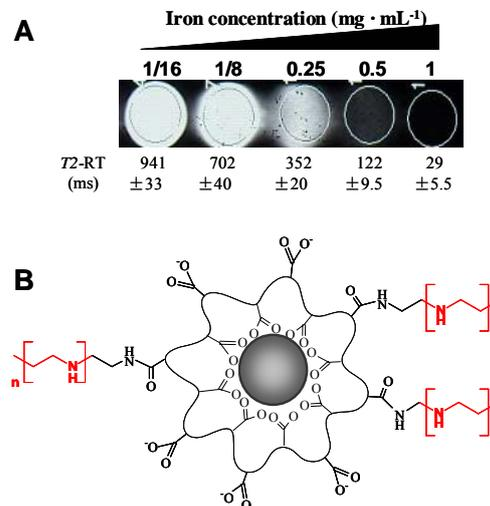
**Figure 1.** (A)  $T_2$ -weighted MR phantom images and  $T_2$ -RT of the SPION in PBS buffer pH 7.4 at different iron concentrations, (B) schematic illustration of pEI-SPIONs.
