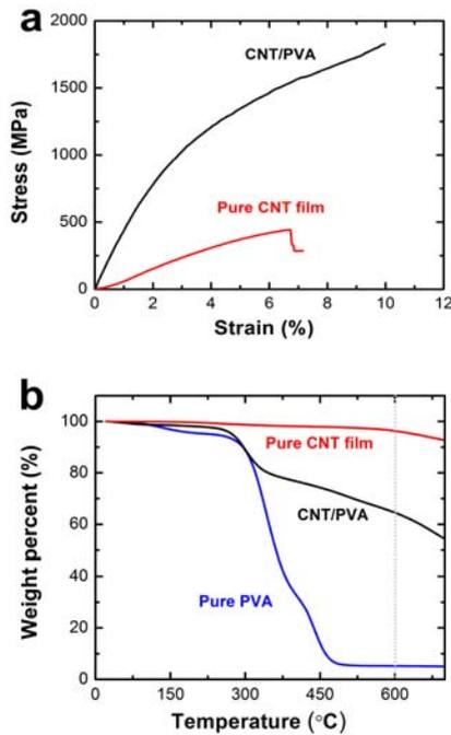
Fig.1 (a) Stress-strain curve of the pure CNT film and CNT/PVA composites; (b) TGA curve of the pure CNT film, CNT/PVA composites and pure PVA.
