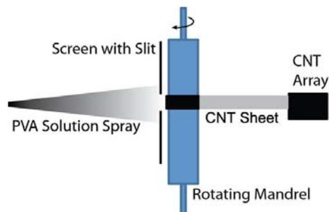
Figure 1: Schematic view of spray winding.
