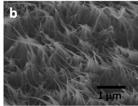
Fig. 3 (a) SEM image of the CNT/PVA composites side view; (b) SEM image of the fracture surface of the CNT/PVA composites.
