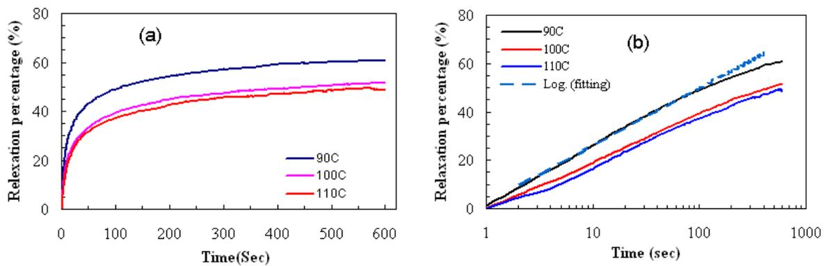
Fig.4: stress relaxation of the SMPC samples extended at 100% with strain as a parameter in linear (a) and semi-log scale (b).
