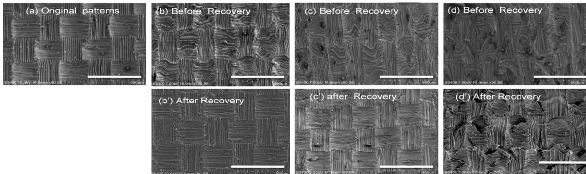
Fig.2 SEM pictures of SMPCs. The upper row are samples strained at 0, 50, 100 and 150% strained at 100 °C, and the lower row are the extended samples recovered after heating at 110°C for 5 mins. White bars are 500 μm scale for all.
