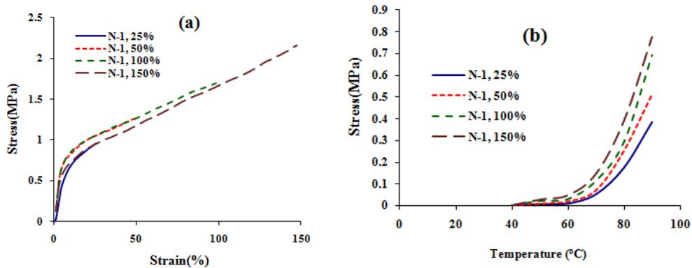
Fig.3a and b: SMPC extended at 90°C at different strains, as per deformation recovery stress generated by individual SMPC samples respectively.
