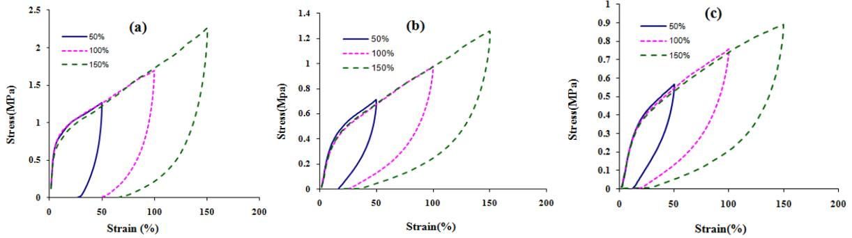
Fig.1: Stress/Strain relationship at strain of 50%, 100% and 150% tested at 90 (a) 100 (b) and 110°C (c) respectively.
