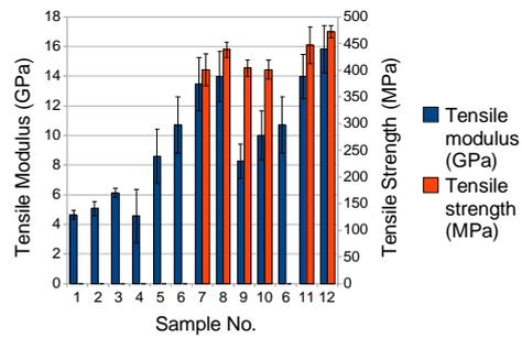
Figure 2: Tensile properties of laminates
