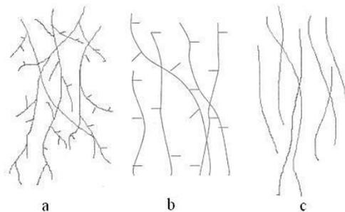
Figure 1: Structure of a) LDPE, b) LLDPE, c) HDPE/UHMWPE
