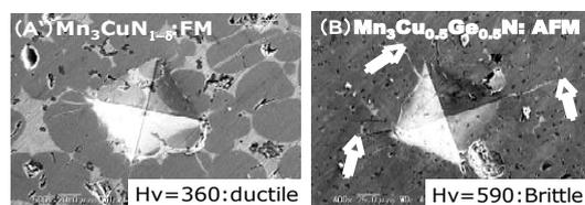
Figure 1: Top view of the Vickers indentation trace of (A)  $\text{Mn}_3\text{CuN}_{1-\delta}$  and (B)  $\text{Mn}_3\text{Cu}_{0.5}\text{Ge}_{0.5}\text{N}$  ceramics. Radial cracks observed in  $\text{Mn}_3\text{Cu}_{0.5}\text{Ge}_{0.5}\text{N}$  are marked with white arrows.
