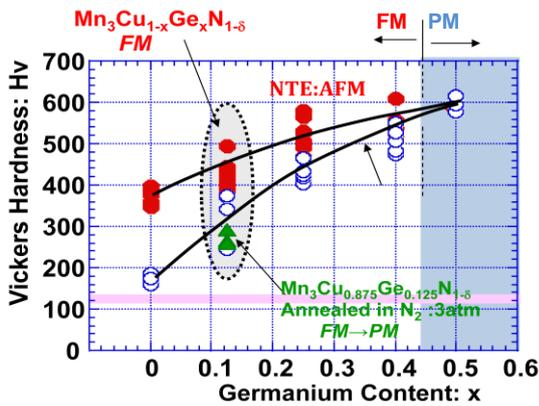
Figure 2: Vickers hardness: Hv as a function of germanium content:  $x$  of  $Mn_3Cu_{1-x}Ge_xN$  (PM: Paramagnetic Metal) and  $Mn_3Cu_{1-x}Ge_xN_{1-\delta}$  FM: Ferromagnetic Metal). At  $x=0.5$ , both  $Mn_3Cu_{1-x}Ge_xN$  and  $Mn_3Cu_{1-x}Ge_xN_{1-\delta}$  specimens are PM at room temperature.
