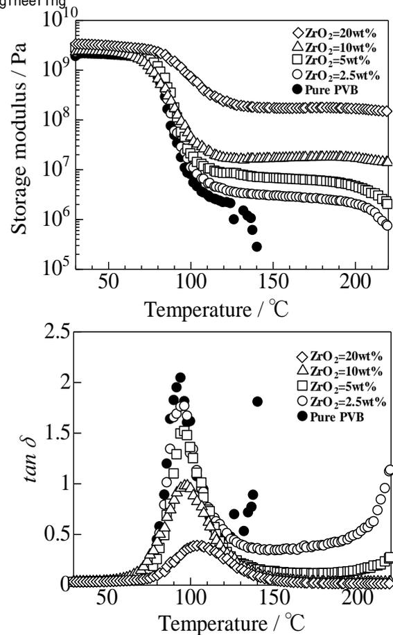
Figure 4 Thermo mechanical spectra of PVB-zirconia hybrids.
