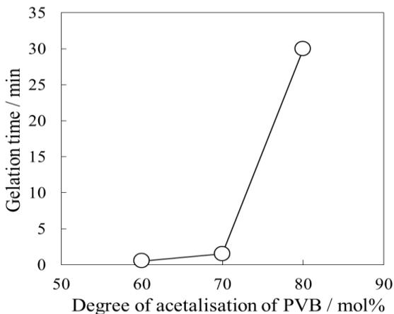
Figure 2 Effect of degree of acetalisation of PVB in PVB/zirconia (90/10 wt.%) mixed solution on gelation time.
