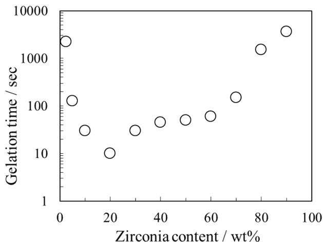
Figure 1 Effect of zirconia content in PVB/zirconia mixed solution on gelation time.
