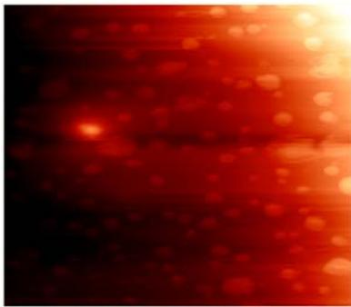
**Fig.1.** AFM of a PEDOT+nc-TiO<sub>2</sub> composite film.
