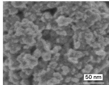
**Fig. 3.** FE-SEM photograph of a MEH-PPV+nc-TiO<sub>2</sub> film with 25 wt% of nc-TiO<sub>2</sub>.
