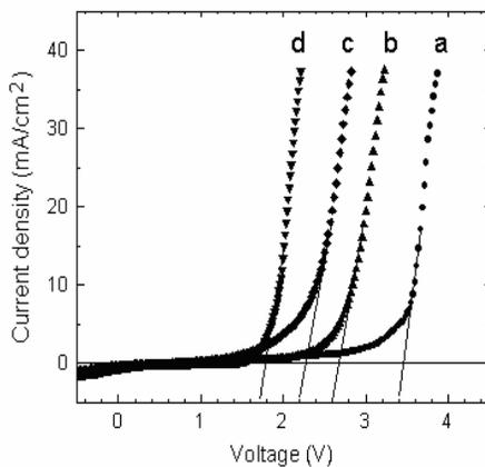
**Fig. 2.** I-V characteristics of OLED with different laminated structure. (a) – Single MEH-PPV; (b) – with HTL layer, (c) – with HTL and EL composite layers, and (d) – With super thin LiF.
