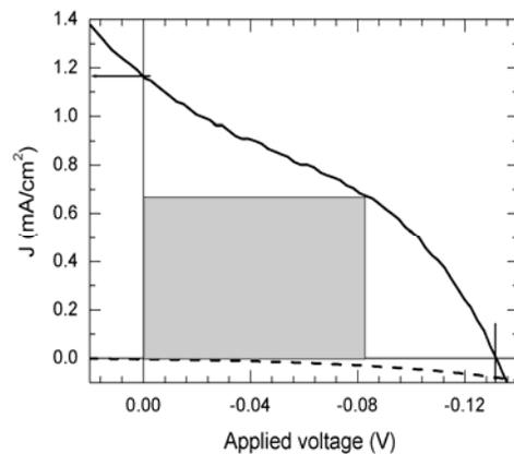
**Fig. 4.** I-V characteristics of a OSC: Thickness the TiO<sub>2</sub> layer is of 30 nm, the MPT composite film – 300 nm and the Al electrode – 100 nm. Pin = 50 mW/cm<sup>2</sup>, Voc = 1.15 V, Jsc = 0.125 mA/cm<sup>2</sup>, FF = 0.34, PEC = 0.15.
