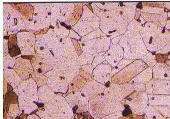
Figure 1: The microstructure of etched fracture plates sintered at 1390°C
