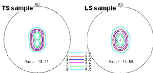
Fig. 4. {00.2} pole figure representing the texture of AZ31 after 60% rolled TS and LS sample at 300 °C
