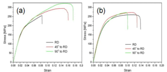
Fig. 5. σ-ε curve for RD, 45° to RD, and 90° to RD, 60% rolled TS sample (a) and LS sample (b)
