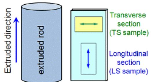
Fig. 1. Samples for rolling, sheets are cut out with a 3mm thickness in a longitudinal section (LS) and transverse section (TS) to the extrusion direction (arrows indicate the rolling direction of sheets)
