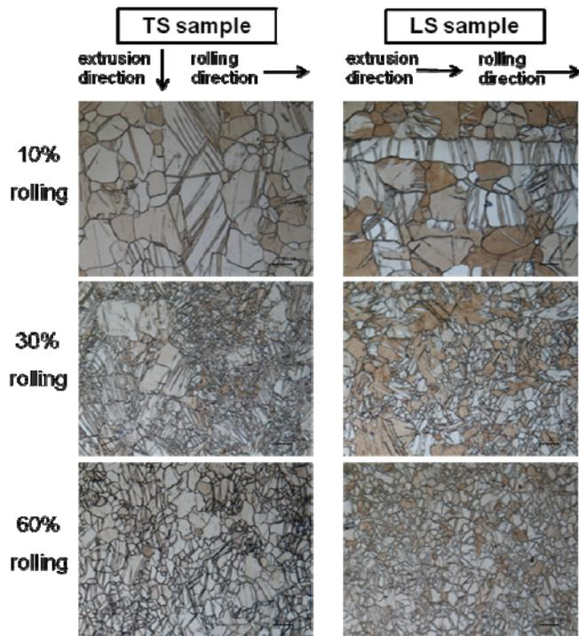
Fig. 3. Microstructure of 10% and 60% rolled TS and LS sample at 300 °C
