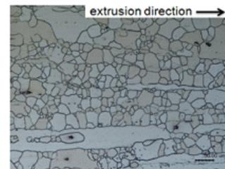
Fig. 2. Microstructure for the longitudinal section of the extruded rod, after full annealing treatment
