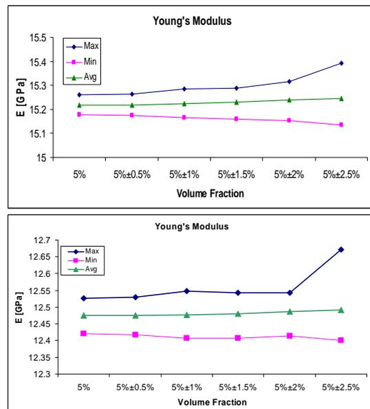
Fig. 2: Young's modulus of CNTRP with straight CNT (top) and non-straight CNT (bottom)
