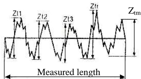
Fig. 1 Used surface measuring parameter - arithmetical middle height [2]
