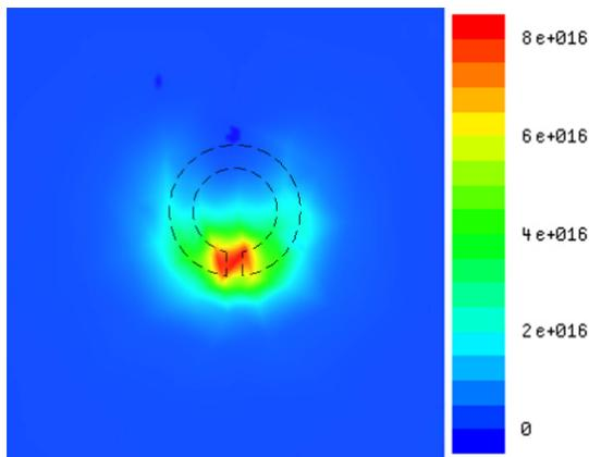
Fig.3. Plot of the total field intensity in the plane 30 nm above the glass surface ( $z=30\text{ nm}$ ).
