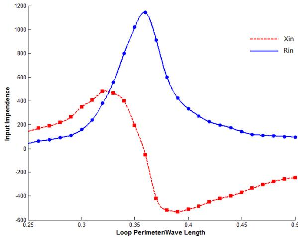
Fig. 2 Simulated input impedance of a nano-loop antenna.
