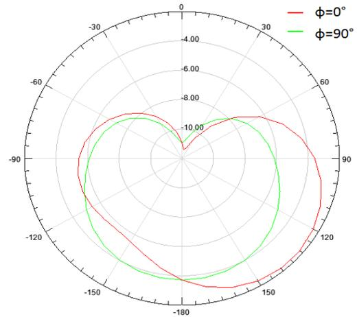
Fig.4. Radiation patterns of the loop antenna in the  $\phi=0^\circ$  plane ( $xz$ -plane) and  $\phi=90^\circ$  plane ( $yz$ -plane).
