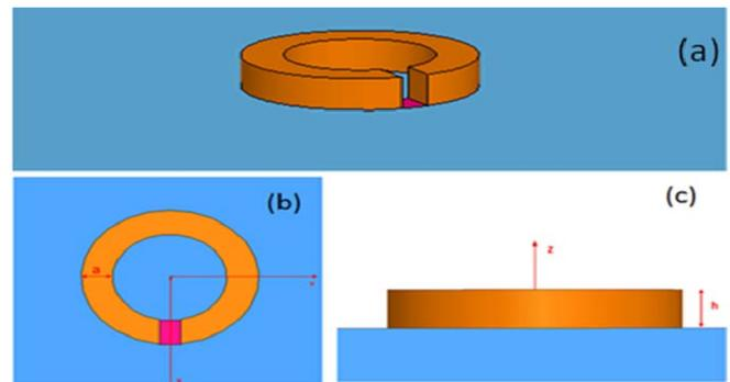
Fig. 1 Sketch of the proposed nano-loop antenna (a) and of its top-view (b) and side-view (c).
