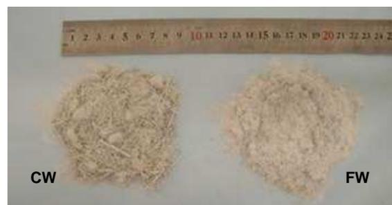
Fig. 1. Coarse (CW) and fine (FW) pultrusion waste.
