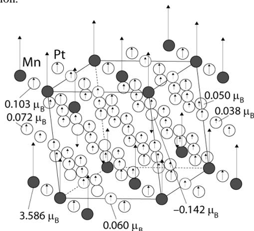
Fig. 3. An alternative ferromagnetic ordering of the  $\text{MnPt}_{15}$  structure in the configuration "base-centered". The Pt atoms at the centers of the faces of the  $2 \times 2 \times 2$  supercell screen the magnetic moments of Mn atoms.
