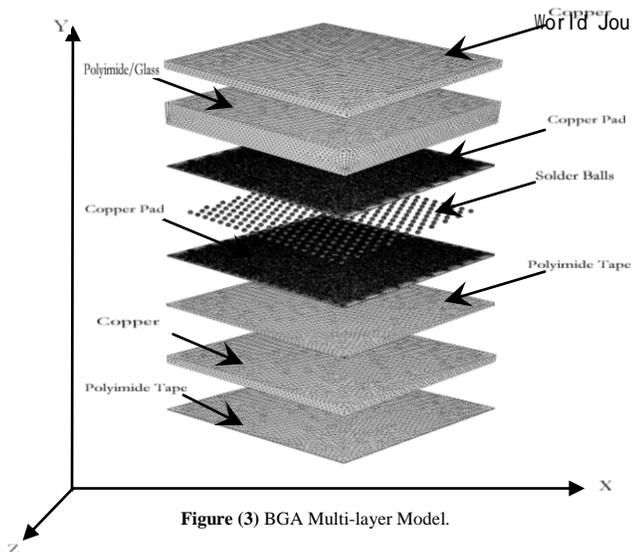
Figure (3) BGA Multi-layer Model.
