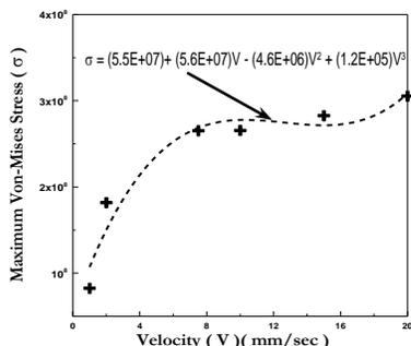
Figure (5) The relation between the impact velocity and the maximum Von Mises stresses at the moment of impact.
