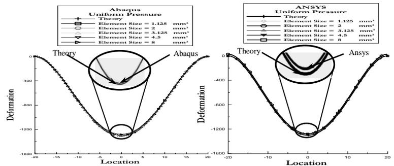
Figure (2) The relation between the location and the deformation in case of the uniform pressure loading condition using Abaqus & Ansys.
