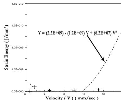
Figure (6) The relation between the impact velocity and the Strain energy.
