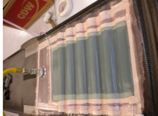
Fig. 2 Patch preparation for secondary bonding or bolting application.
