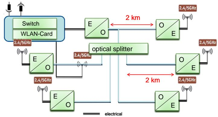
Fig. 5 Trainguard MT Metro Shanghai RoF-WLAN Transmission System
