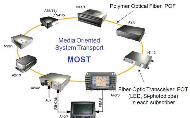
Fig. 2 MOST network with ring topology developed using optoelectric (O/E) and electrooptic (E/O) components for transmitters and receivers as well as a fiber in the center of the arrangement (Fig.1). These
