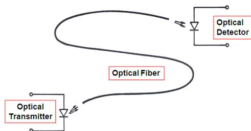
Fig. 1 – Basic arrangement of a fiber-optic system
