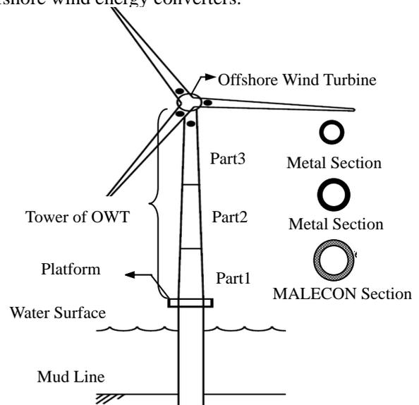
Fig. 2 Concept of hybrid tower
