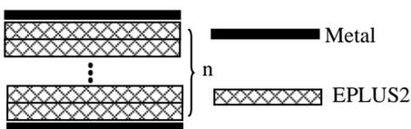
Fig. 1 Concept of fiber-metal laminates-MALECON
