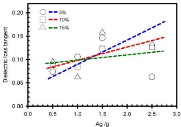
Fig. 2 The dielectric loss tangent of the PMMA/Fe<sub>3</sub>O<sub>4</sub>NP/AgNP composites.
