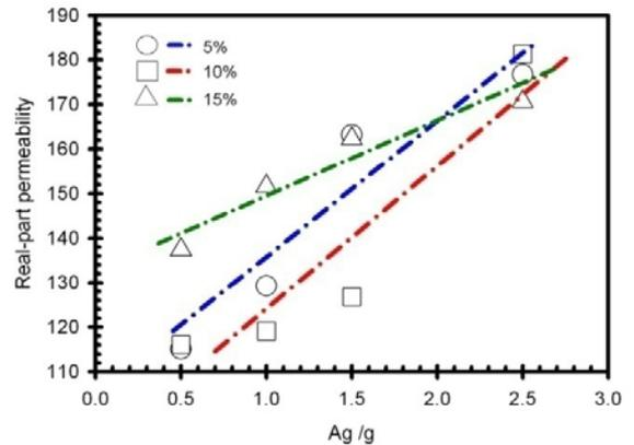
Fig. 3 The real-part permeability of the PMMA/Fe<sub>3</sub>O<sub>4</sub>NP/AgNP composites.
