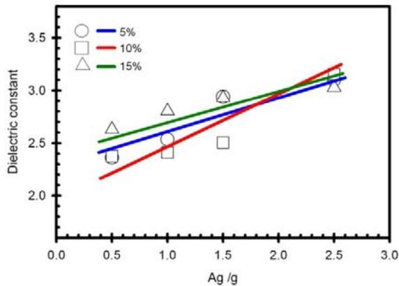
Fig. 1 The dielectric constant of the PMMA/Fe<sub>3</sub>O<sub>4</sub>NP/AgNP composites.
