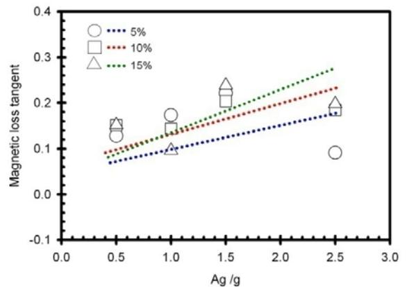
Fig. 4 The magnetic loss tangent of the PMMA/Fe<sub>3</sub>O<sub>4</sub>NP/AgNP composites
