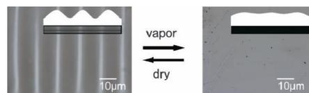
**Fig. 2.** Optical microscopy images of long-range ordered surface wrinkles before (left image) and after water vapor treatment (right image). In the insets, a sketch of the surface change during the process is depicted.
