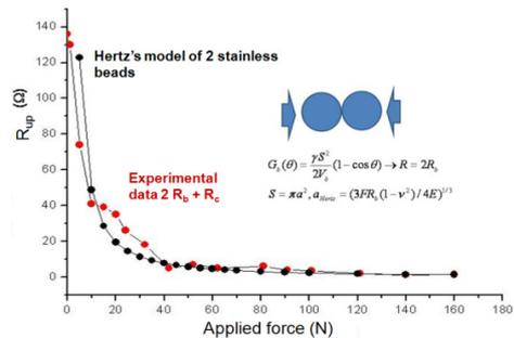
Figure 4: Effect of the applied force on the beads resistance
