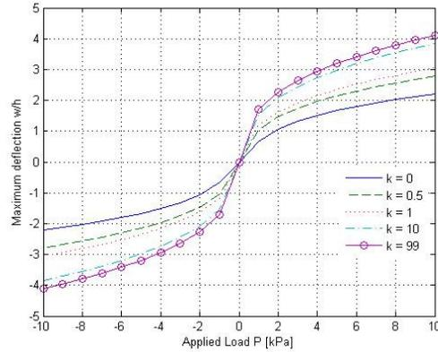
*Maximum deflection of the beam under cylindrical bending with various k values*
