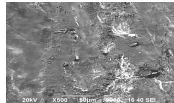
Fig 5: Worn out surface of the thermally oxidised sample after the sliding wear test
