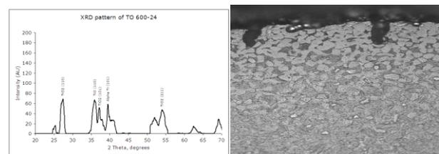
Fig 1(a): X-Ray Diffraction pattern (b): Microstructure of the sample oxidised at 600°C for 24 hours
