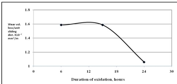
Fig 3: Variation of wear volume loss/unit sliding distance with the duration of thermal oxidation
