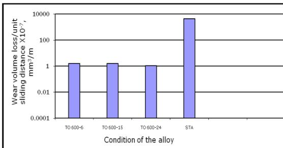
Fig 4: A comparison of the wear volume loss in various thermal oxidation conditions with that for a sample in STA condition
