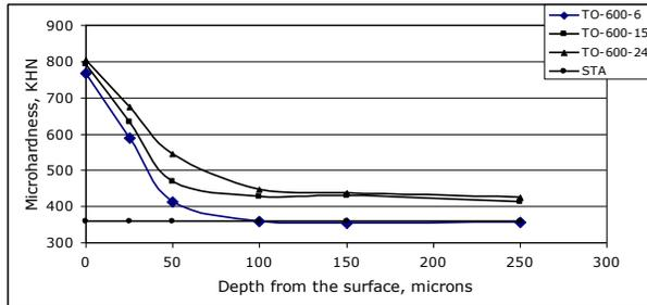
Fig 2: Microhardness-depth profile of the samples oxidised at 600°C for different durations
