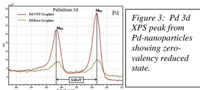
Figure 3: Pd 3d XPS peak from Pd-nanoparticles showing zero-valency reduced state.
