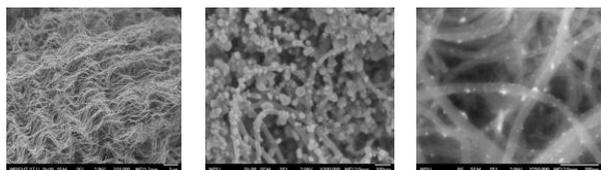
Figure 1: SEM images of (a) carbon nanotube (CNT) (b) Pd-CNT and (Ag-CNT structures.
