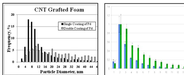
Figure 2: Particle Size distributions of (b) Pd on CNT and (b) Ag on CNT.
