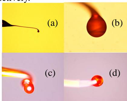
Fig. 2. (a) Microscope image of a chalcogenide fibre with a taper-drawn and a microsphere at the end of taper, three
