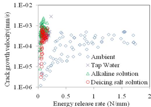
Fig. 2 Subcritical debonding of epoxy-concrete interface in different environments
