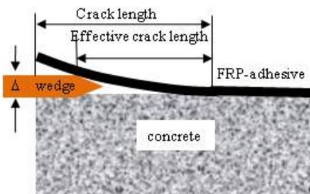
Fig 1 Wedge-driven specimen
