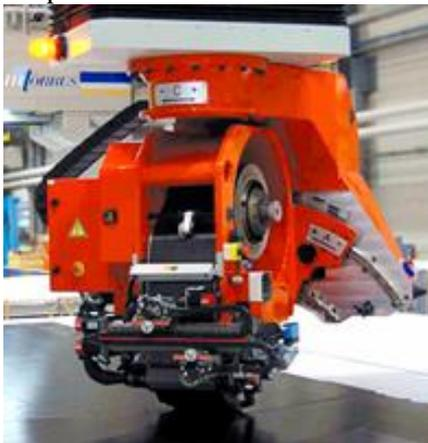
Fig. 1: Automated tape laying head
