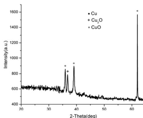
Fig. 3 XRD pattern of 1 μm copper film annealed at 400 °C in air for 4h.
