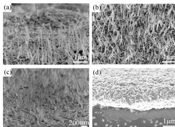
Fig. 1 SEM cross-sectional images of 1μm thick copper films annealed at 400°C in air for different annealing time: (a) 2h, (b) 4h, (c) 5h, and (d) 6h.
