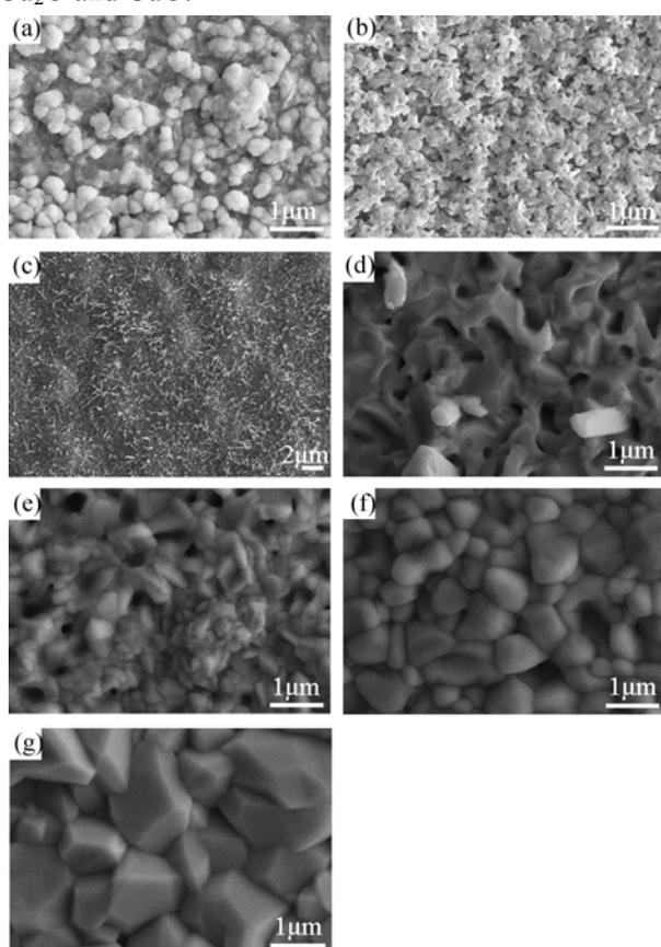
Fig. 2 SEM images of 1 μm thick copper films annealed for 4h in air at various temperatures: (a) 300 °C, (b) 350 °C, (c) 400 °C, (d) 450 °C, (e) 500 °C, (f) 600 °C, and (g) 700 °C.
