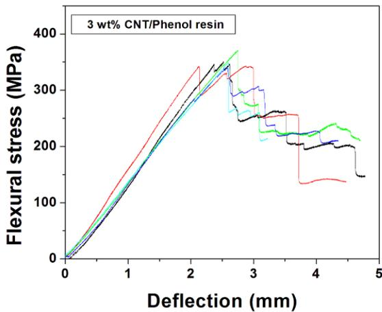
Fig. 2 Flexural stress of carbon fabric-phenolic resin composites reinforced by 3 wt% CNTs.
