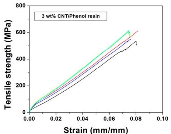
Fig. 1 Tensile strength of carbon fabric-phenolic resin composite reinforced by 3 wt% CNTs.
