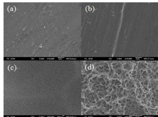
Fig.1 Morphologies of untreated (a), polished (b), anodized in H<sub>3</sub>PO<sub>4</sub> (c) and HF (d) NiTi wires
