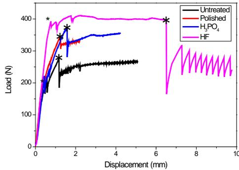
Fig. 2 Typical load vs. displacement curves of pullout test
