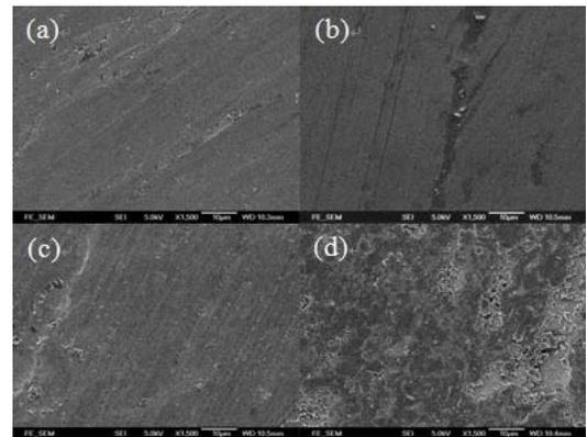
Fig. 3 The fracture surface of fibre pullout test: (a) untreated; (b) polished; (c) anodized in  $H_3PO_4$ ; (d) anodized in HF
