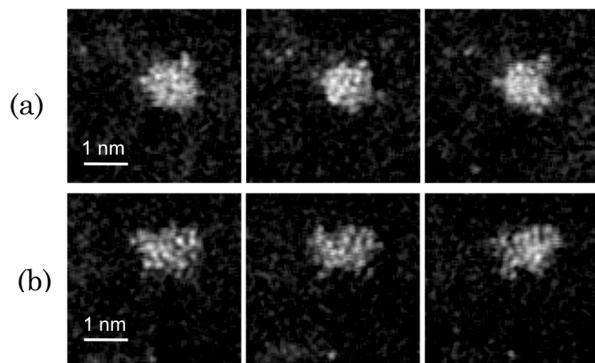
Fig. 2 Representative series of HAADF images (0.2 s/frame) under optimized experimental conditions. (a) shows a cluster with circular projected shape and an aspect ratio of 1.08; (b) shows a cluster with a prolate projected shape and an aspect ratio of 1.52.
