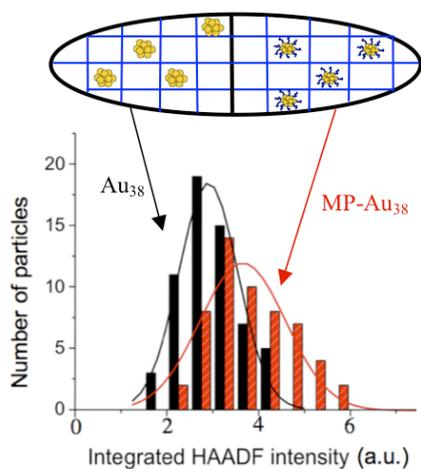
Fig. 1 Statistical integrated HAADF intensities obtained for size-selected Au<sub>38</sub> clusters and MP-Au<sub>38</sub> clusters which were co-deposited on the same TEM grid.
