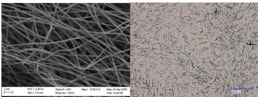
Fig. 4 a) C-Nanofibers and b) Dispersion in rubber
