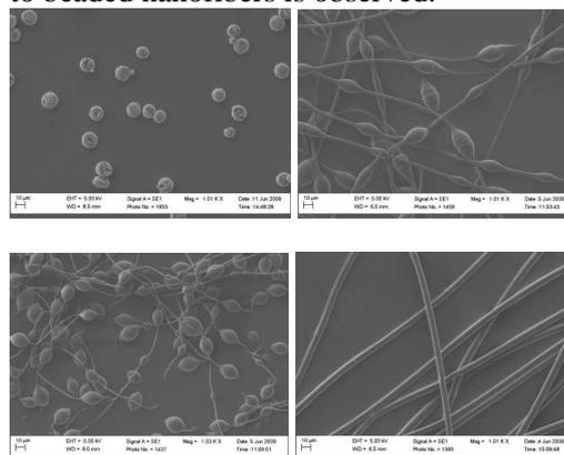
Fig. 1 Influence of polymer concentration on the morphology of electrospun fibers
