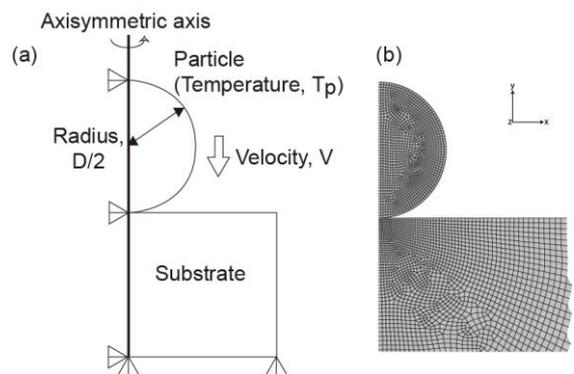
Fig. 2 Schematic of analysis model: (a) a particle impacting on a substrate, (b) typical finite element mesh used in the simulation.
