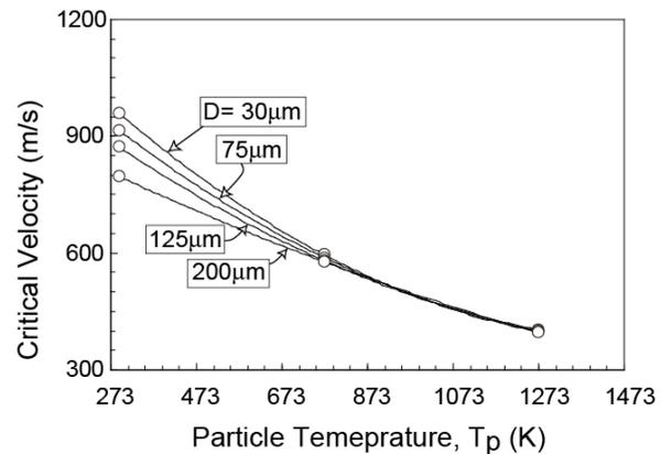
Fig. 4 Effect of particle size on the critical velocity of a titanium particle impacting on a titanium substrate.
