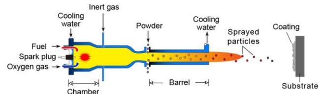
Fig. 1 Schematic of Warm Spray deposition.
