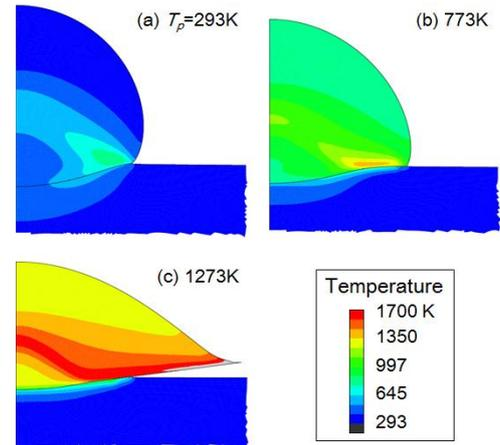
Fig. 3 Variation of particle deformation and temperature distribution at 200 ns after impact.
