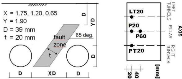
Fig. 4 Experimental models – parametric study (left), measurement points at the model surface (right)
