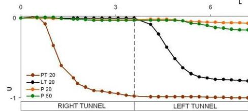
Fig. 7 U-L diagram for excavation of the right and then left tunnel (without fault zone, 1.75D)
