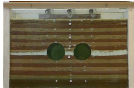
Fig. 2 Physical model Geo-Brno 2010 after finishing the building of the model
