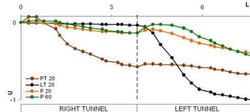
Fig. 8 U-L diagram for excavation of the right and then left tunnel (with fault zone, 1.75D)
