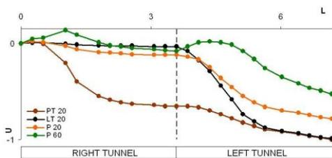
Fig. 5 U-L diagram for excavation of the right and then left tunnel (without fault zone, 0.65D)
