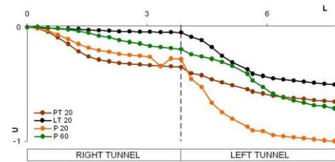
Fig. 6 U-L diagram for excavation of the right and then left tunnel (with fault zone, 0.65D)
