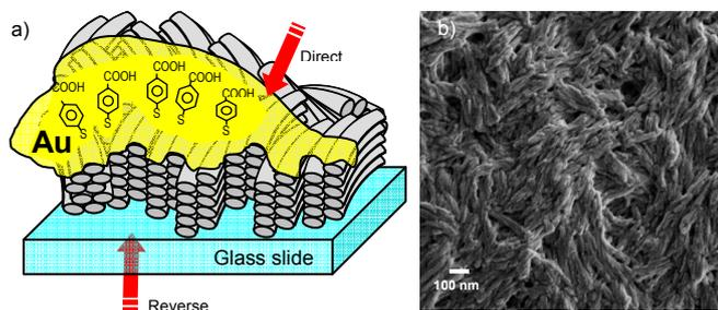
Fig. 1 a) Preparation of glass slides with sandwiched 4-MBA/Au/cross-linked  $\beta$ -ICD amyloid layers for SERS measurements. The red arrows indicate two directions of the backscattered incident laser beam examined in this study: direct and reverse. b) The corresponding SEM image obtained after sputtering amyloid fibrils with Au/Pd.
