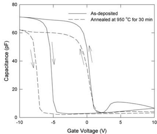
Fig.4. C-V characteristics of MOS capacitors showing the hysteresis due to charge localization in dielectric traps or embedded silicon nanoparticles.
