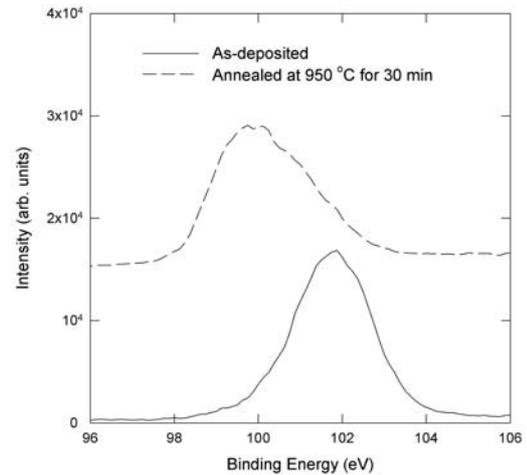
Fig.3. Si 2p XPS spectra for as-deposited and high-temperature annealed silicon nitride films.
