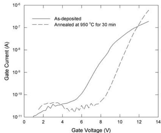
Fig.5. Current-voltage characteristics of MOS capacitors with different gate dielectric films.
