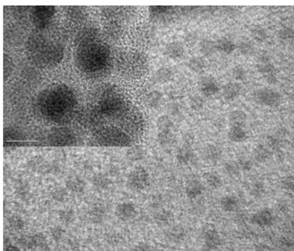
Fig.2. TEM micrograph showing the silicon nanoparticles embedded in a silicon nitride film.
