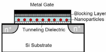
Fig.1. Structure of flash memory cell based on silicon nitride embedded silicon nanoparticles.
