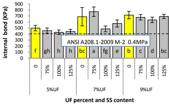
Fig.2. Internal bond strength of particleboard
