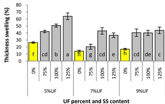
Fig.1. Thickness swell after 24H soaking of particleboard (means with the same letter are not significantly different at the 5% probability level, the following figures are also).
