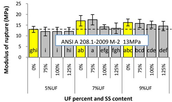
Fig.4. Modulus of rupture (MOR) of the particleboard
