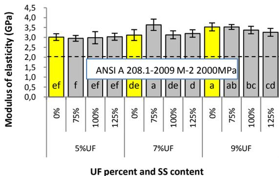
Fig.3. Modulus of elasticity (MOE) of the particleboard
