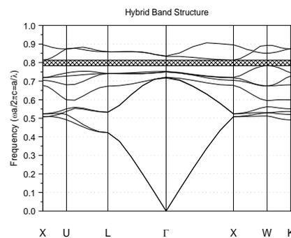
Fig 3 Simulated photonic band structure of silicon inverse opal.
