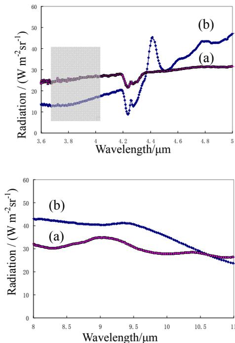
Fig 2 Radiation spectra of silicon inverse opal(a) and bulk silicon wafer (b)
