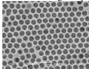
Fig 1 SEM image of a silicon inverse opal. Emission measurements were performed by heating silicon inverse opals to ca.  $250^\circ\text{C}$  in an ambient atmosphere. The emission spectra of silicon inverse opal on flat silicon substrate
