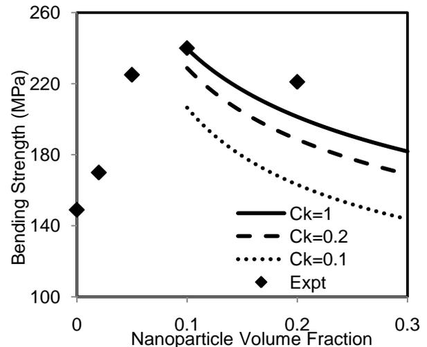
**Figure 1.** Variation of the nanocomposite bending strength with the nanoparticle volume fraction. Data from Soh et al [6].
