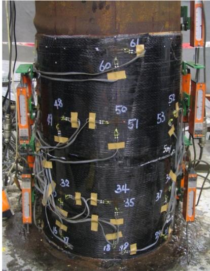
Figure 1. Failure mode of a confined CFST with a 6-ply CFRP jacket
