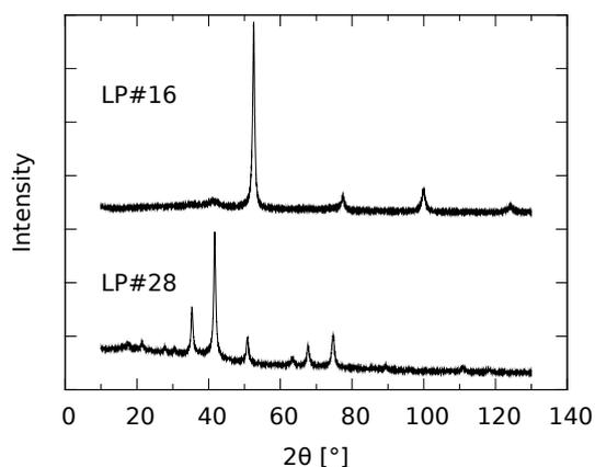
Fig. 2: XRD analysis of both samples.
