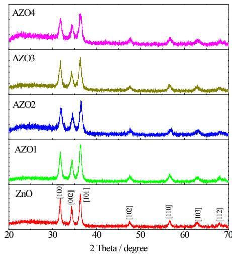
Fig. 1 XRD patterns of the ZnO and AZO1~4 NCAs.
