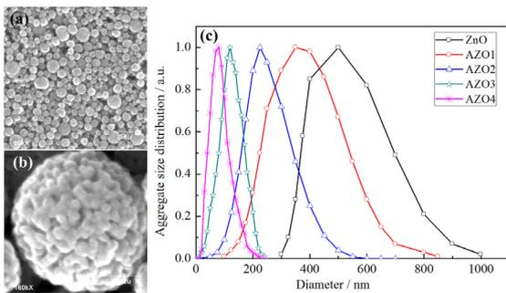
Fig. 2 SEM images of the AZO4 NCAs (a) low-magnification image, (b) high-magnification image and (c) particle size distribution curves of the ZnO and AZO1~4 NCAs.
