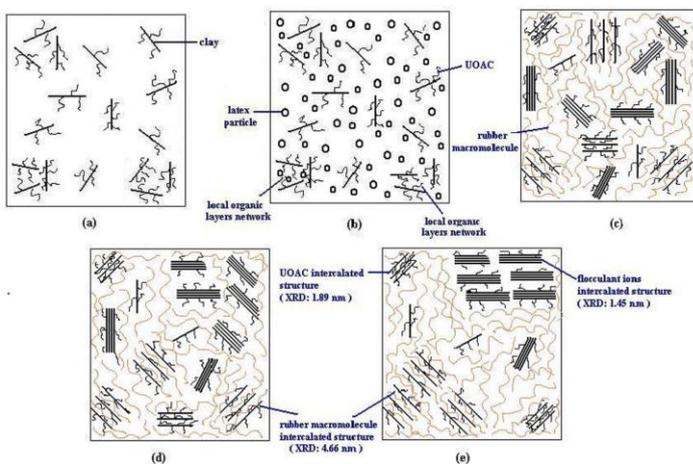
Na<sup>+</sup>-MMT was modified organically in situ in its aqueous suspension by controlling the amount of modifier, an UOAC, to prevent clay aggregation. SBR latex and the modified MMT aqueous suspension were mixed to prepare organically modified MMT-SBR nanocomposites by the LCM method. The dispersion structure of nanocomposites by this new strategy can be defined as a "separated structure" with part
