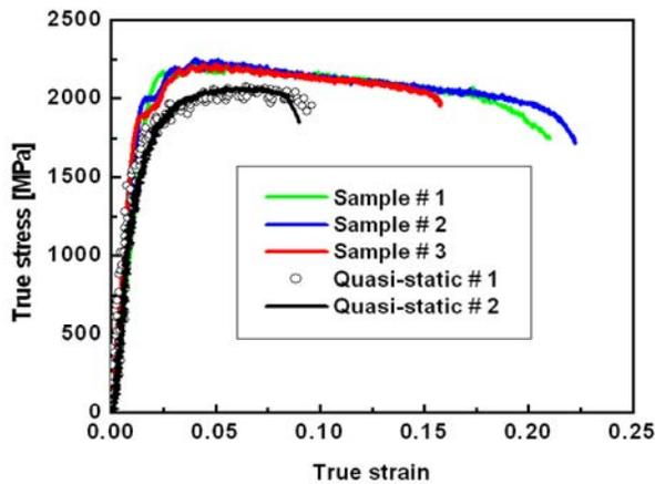
Fig. 2 Dynamic and quasi-static true stress-strain curves of the nanocrystalline NiFe alloy [7]. Three samples were used for the dynamical tests with strain rates ranging from  $1 \times 10^3 \text{ s}^{-1}$  to  $3 \times 10^3 \text{ s}^{-1}$ . Significantly enhanced dynamic deformation strain and strength were observed compared to the quasi-static loading with a strain rate of  $1 \times 10^{-3} \text{ s}^{-1}$ .
