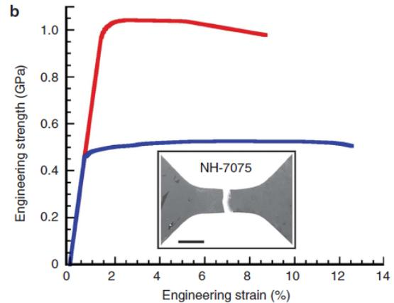
Fig. 3 Engineering stress-strain plot for the nanocrystalline (NH) 7075 and T6-7075 alloy [8]. The inset is the fractured tensile specimen of the HN-7075 Al alloy.
