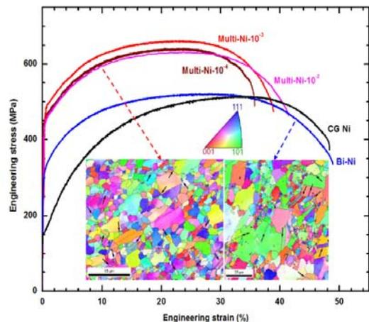
Fig. 1 Tensile engineering stress-strain curves of multi- (Multi-Ni) and bi-modal (Bi-Ni) Ni samples prepared by cryomilling and quasi-isostatic forge [6]. The CG Ni was achieved by annealed the multi-Ni sample at 1000 °C for 10 h.
