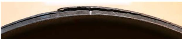
Fig. 4 A failed flexure control specimen
