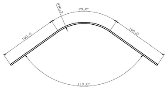
Fig. 1 Dimensions of beam specimen
