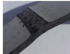
Fig. 2 Removed crest of a crease
