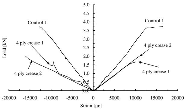
Fig. 3 Load-strain curves for creased and control specimens in flexure tests
