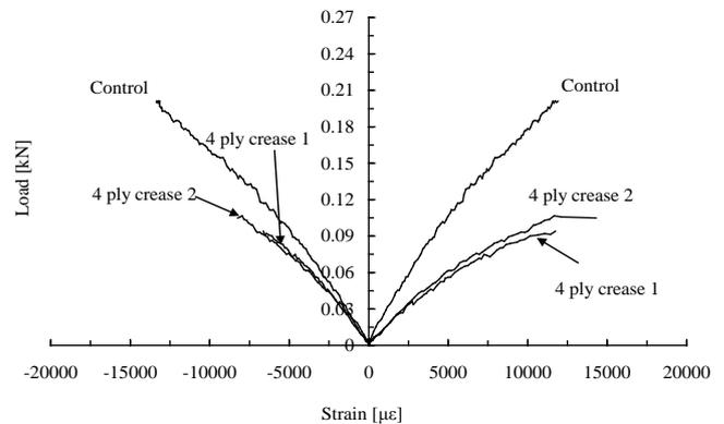
Fig. 6 Load-strain curves for control and creased specimens in compression test
