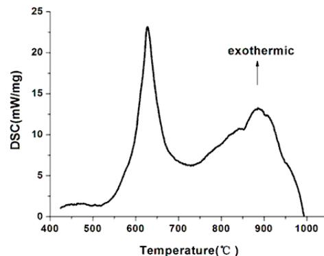
Fig.2 DSC plot of as-deposited Al/CuO RMFs.
