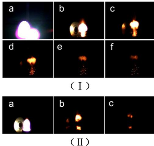
Fig.3 High speed camera observation of electrical explosion process at 600V: ( I ) images of Cu/Al/CuO RMFs. ( II ) images of Cu film.
