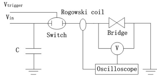
Fig.1 Schematic drawing of the test circuit.
